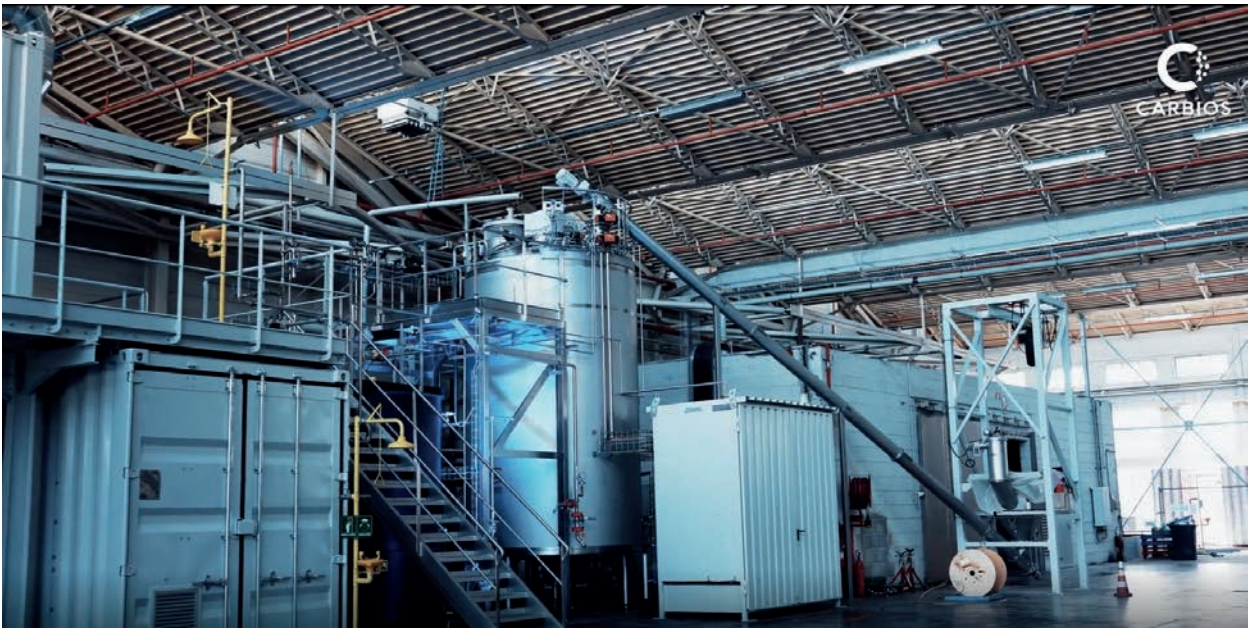
Enzymatic hydrolysis reactor for the depolymerization of PET plastic and textile waste into monomers (credit: Carbios)
