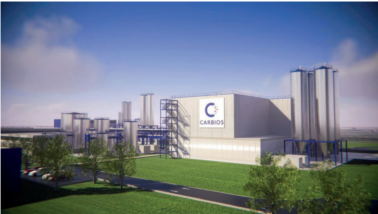
3D modeling of the Carbios industrial unit for the depolymerization of PET plastic and textile waste into monomers (credit: Technip Energies)
